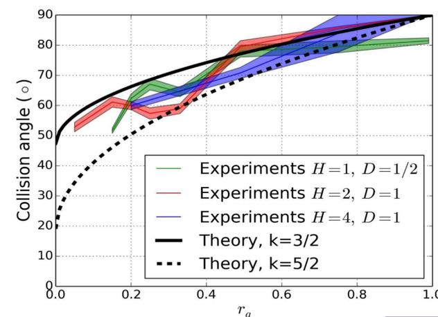
Figure 4. Comparison between the theoretical values for the angle given by the formula and numerical values.
