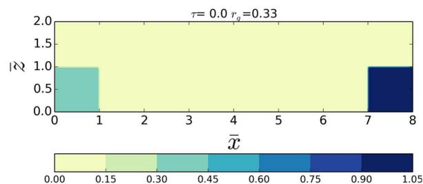
Figure 1. Numerical model domain at initial time. Color bar indicates buoyancy scale.
