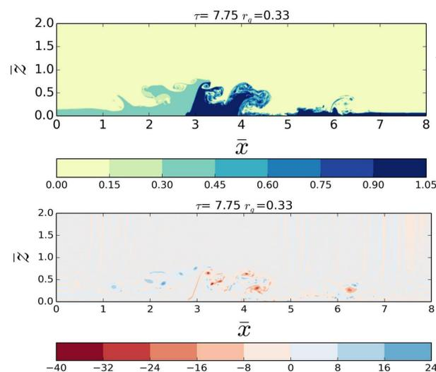
Figure 2. Snapshot of buoyancy (top) and vorticity field (bottom) model output at the moment of collision for experiment 11.
