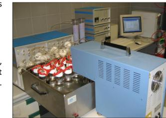
Figure 2. Respirometer Micro-Oxymax, Columbus.
